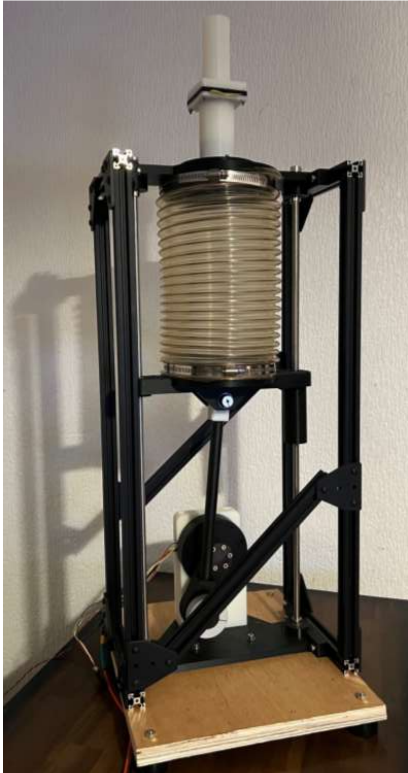
Figure 1. Robotic Lung. Image of the lung apparatus, shown with a simple larynx model attached at the top.
