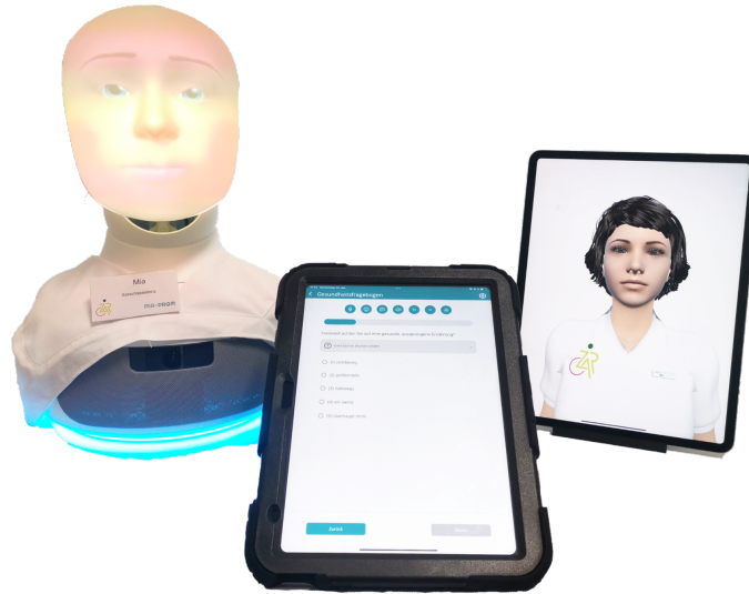
Figure 1 – In MIA-PROM, the system can be instantiated in three distinct configurations: (i) a standalone tablet interface (center), (ii) a tablet interface accompanied by a physical avatar (left), and (iii) a tablet interface accompanied by a virtual avatar (right).
