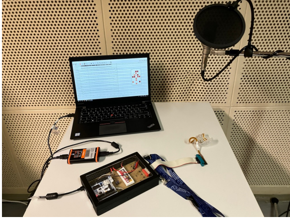
Figure 3 – Recording setup: laptop with ADR2, OPG2023 and microphone.
