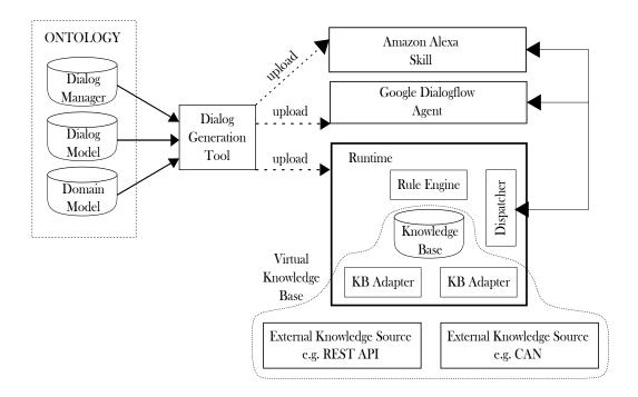
**Figure 1** – Overview of the architecture: The ontology is converted to a knowledge base and uploaded by the Dialog Generation Tool. One part is deployed to Alexa and/or Google to enable speech recognition and semantic analysis. The other part is the knowledge base used by the rule engine. It is uploaded to the server hosting the runtime environment/dialog back-end.
