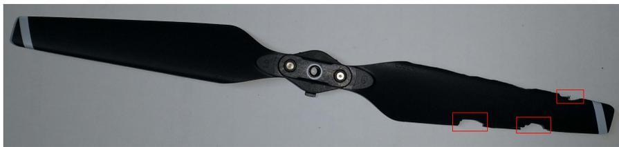
**Figure 4** – Imitated cracks in one of the rotor blades (on the right)
