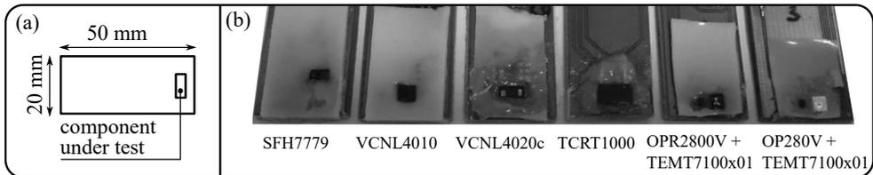
**Figure 3** – (a) Standardized test sensor dimensions and optical component position, (b) examples of tested sensors and their encapsulation.
