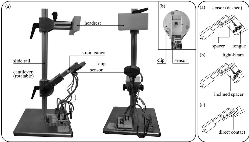
**Figure 2** – Left: (a) Constructed test station. (b) Close-up of a sensor mounted on the sensor clip. Right: Spacer setup for the different measurement quantities. (a) Level spacer placed between sensor and tongue for distance measurements. (b) Inclined spacer for angle measurements. (c) Removed spacer for force measurements.
