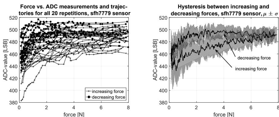
**Figure 4** – Left: measurements of force vs. ADC-value across all 20 repetitions for sensor D3, separated for increasing (+) and decreasing (o) force. Right: mean and standard deviation (calculated as described in Section 4) for the emphasis of the hysteresis between increasing and decreasing forces.
