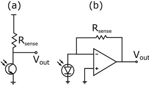
**Figure 1** – Basic circuitry used for the conversion of a photocurrent into a voltage.
