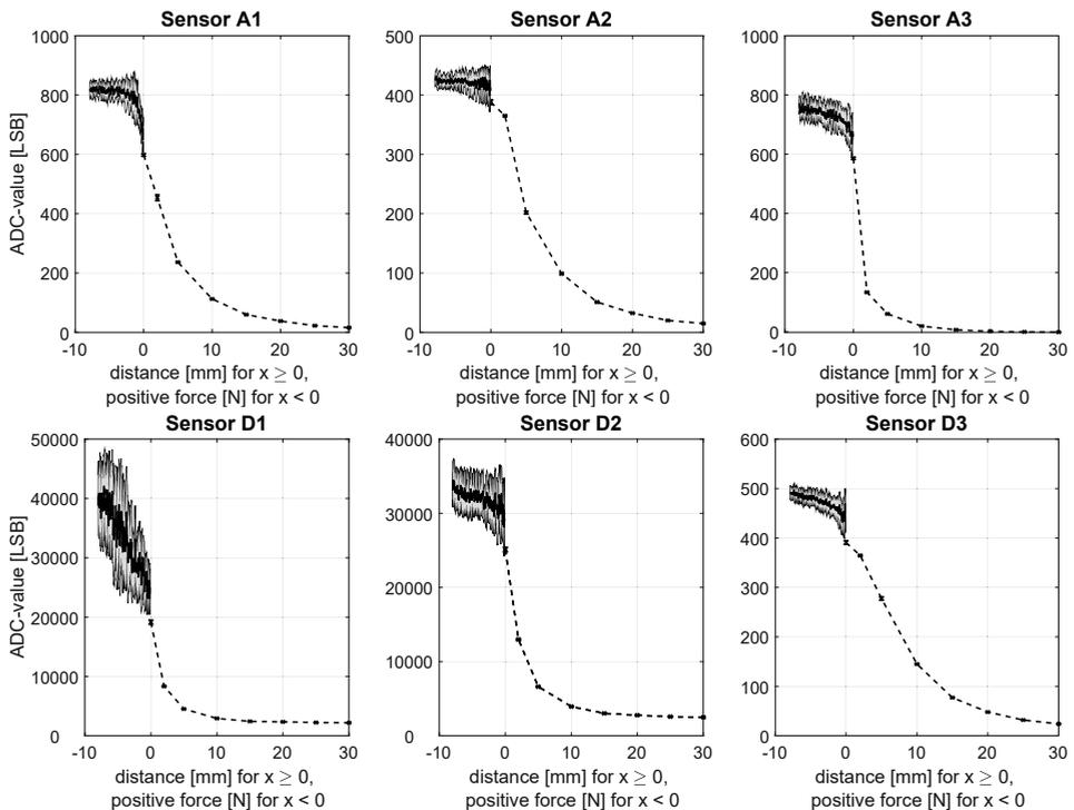
**Figure 6** – Dynamic plots of combined force and distance measurements for all tested sensors.
