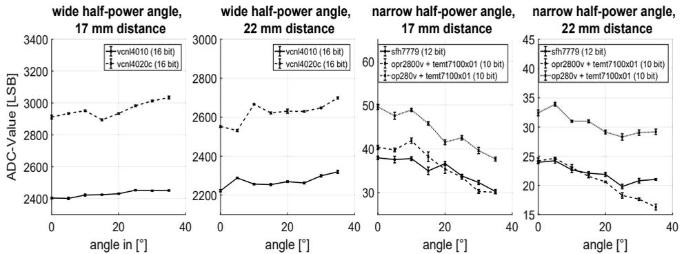
**Figure 5** – Sensor ADC-value over inclination angle. The distance from sensor to tongue is fixed to 17 mm and 22 mm, respectively.
