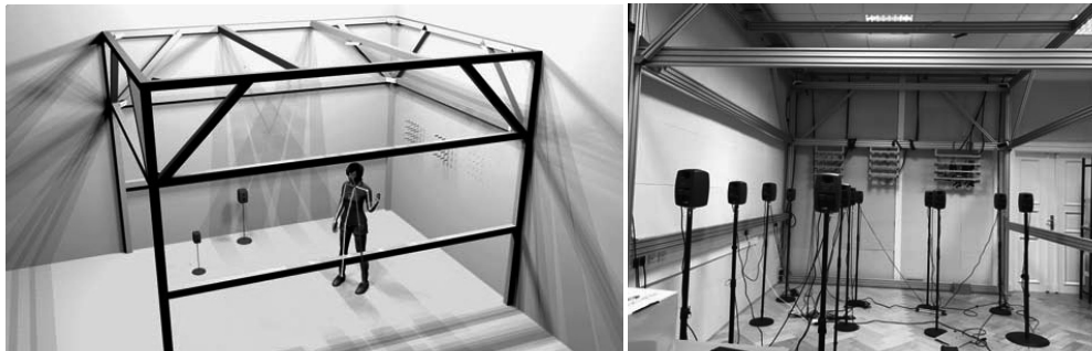
Figure 3 – Laboratory: (left) 3D model with two speakers and one person, (right) experimental setting with multiple speakers and three microphone arrays
