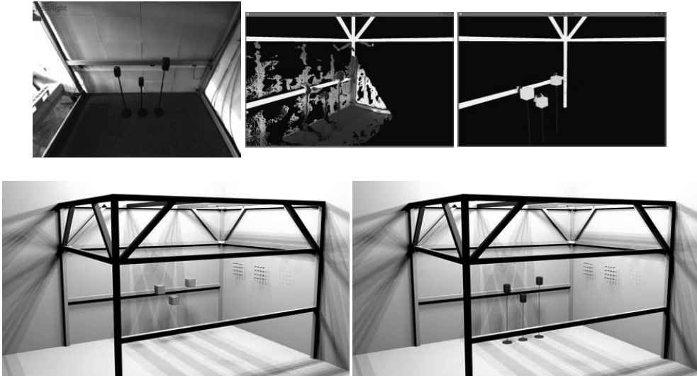
Figure 1 – Example of 3D localisation workflow from top left to bottom right: static objects like speakers localised using point cloud information (for details, see text)
