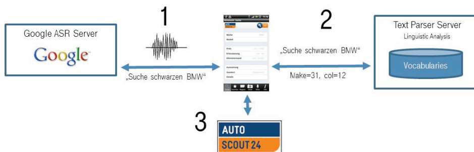
Abbildung 2 - Overview of the general approach.
