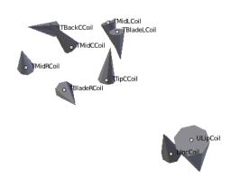
**Figure 2** – Perspective view of EMA coils rendered as primitive cones to visualize their orientation
