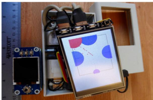
**Figure 1** – A first prototype based on a Raspberry Pi with 4 USB microphones and a display.
