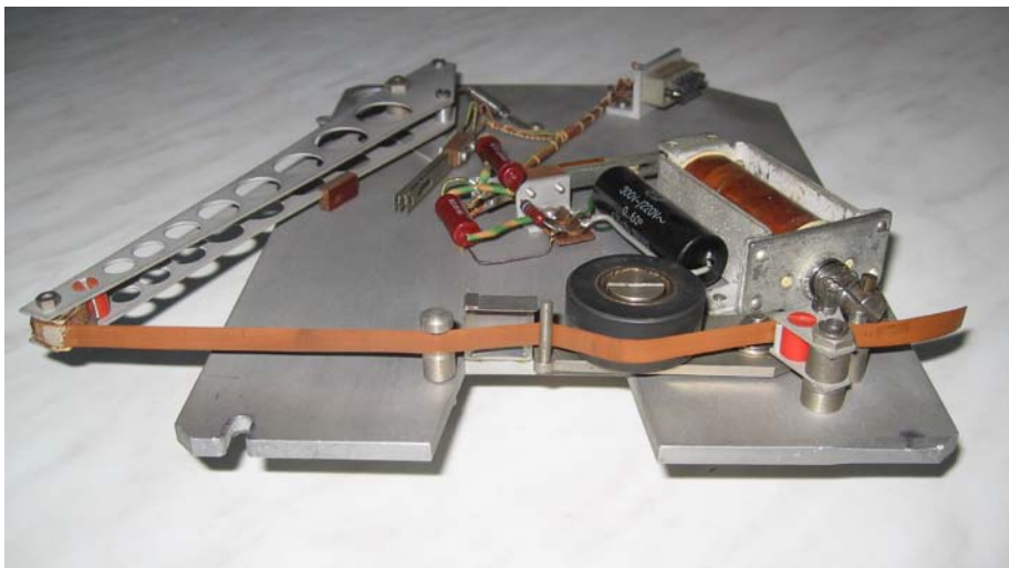
Figure 4 - A single segment of the magnetomechanical speech synthesizer “Lora” from 1964 (FTZ Darmstadt, Germany). One segment served as storage for one spoken sound. From the historic acoustic-phonetic collection of the TU Dresden.
