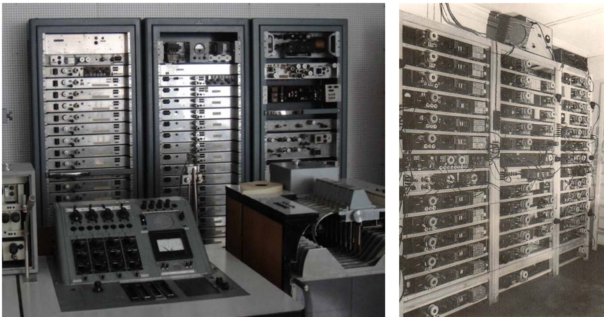
Figure 2 – Historic vocoders in Germany. Left – The Siemens vocoder in the background of the Siemens Studio for Electronic Musik, now in the Deutsches Museum in Munich. Right: Historic photograph of the Dresden vocoder. The left rack contained the analyzer channels, the two right racks the synthesizer channels [8].
