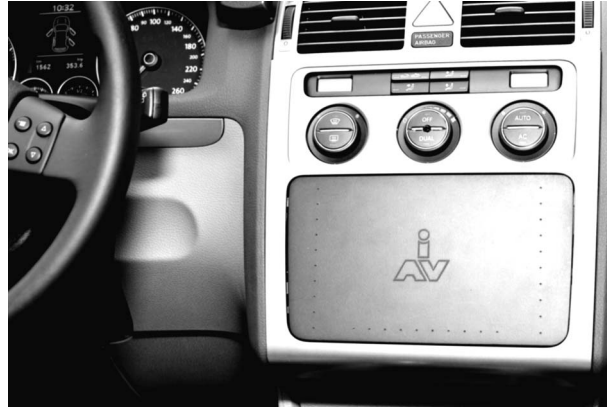
Figure 4 - Head-unit-integrated microphone array with 30 channels for research in a middle-class car.
